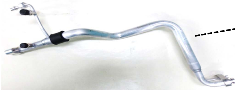
I H X (Internal Heat Exchanger)
