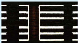
厚銅基板断面 X-section of Heavy-Cu PWB
