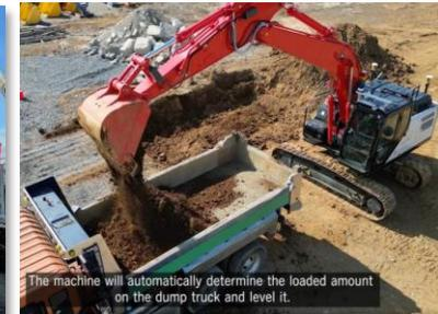
The machine will automatically determine the loaded amount on the dump truck and level it.
