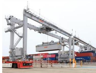
RTG = Rubber Tired Gantry crane
